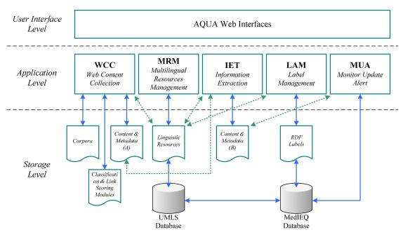
Figure 1. Architecture of the AQUA system.
